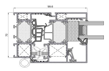
The XP-70 HI system, 70 mm of section and standard canal for eurogroove hardware, has a 34 mm thermal breack and HI thermal insulation in the air chamber, resulting in higher performance.
