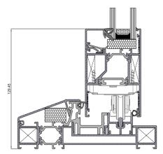
The XS-150 system, designed for balconies and with an innovative closing system, achieves maximum performance in terms of permeability and watertightness. It allows the frame to be fully integrated for free passage between the interior and exterior of the estance.
