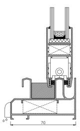
In-line sliding system without thermal breack and 45° cut with simple assembly and design.
