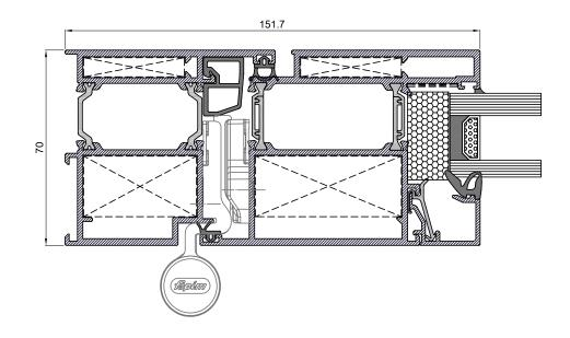
The XD-70 aluminium door system has been designed to meet the requirements of any project in terms of insulation, security and design.
