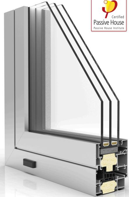
The XP-80 HI system, with 80 mm of section, standard canal for eurogroove hardware, 44 mm thermal break and HI thermal insulation in the air chamber, offers the best thermal and acoustic performance. Due to its properties, it is PassivHaus certified.
