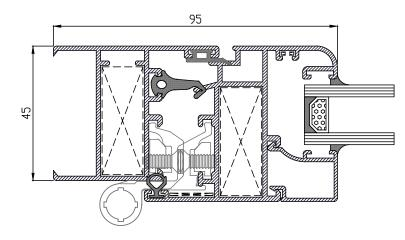
Practicable system without thermal breack and reduced size with 45 mm of frame.
